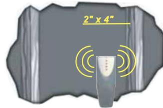
You must attach the TV wall mount to a wall that has at least 2" x 4" wood studs to avoid property damage or injury.
