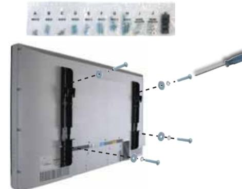
The hooks must be on the top, and the security screws must face the screen edge.
